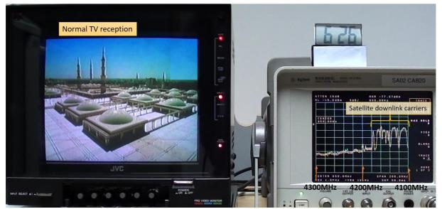
Figure 4: Spectrum plot where a C-band receiver is not affected by aircraft altimeter
