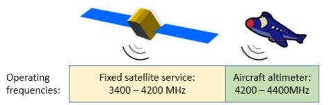
Figure 2: Operating frequencies for fixed satellite service and aircraft altimeter
