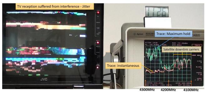
Figure 5: Spectrum plot where a C-band receiver is affected by aircraft altimeter - TV reception: jitter
