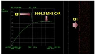
Fig. 3 Spectrogram of Interference B
