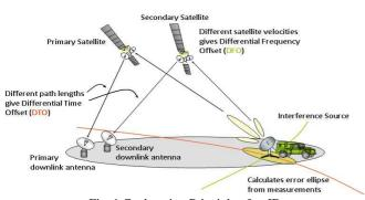
Fig. 1 Geolocation Principle of satID
