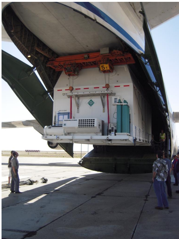
Offloading the AsiaSat 5 spacecraft container at Yubileiny Airfield in Baikonur
